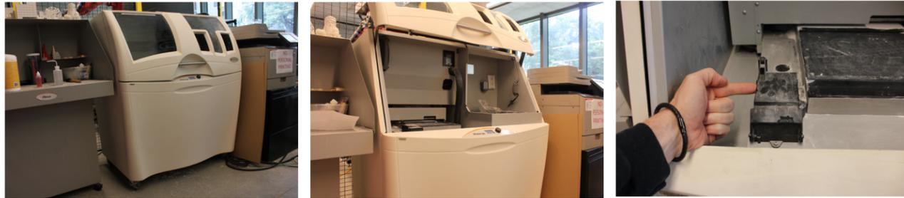
2. Open and empty the reservoir to the left that looks like it has a liquid in it. This liquid is the glue the machine uses to glue the powder in the correct shape. Use a paper towel and soak up the liquid as much as possible. **DO NOT** allow any liquid or powder to get on the piece of cotton on the lower left, this cotton cleans the print head after each layer of glue.
